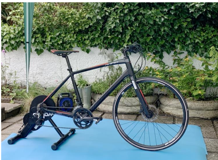
Figure 4.1 Giant Rapid' bicycle mounted on Wahoo Kickr.
