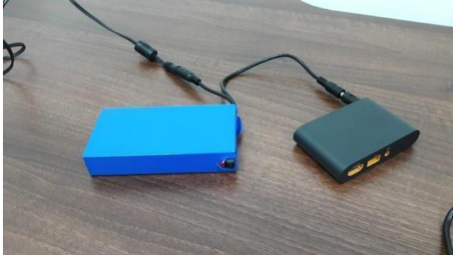
Figure 3.15 Powering the Vive's linkbox using a 12V battery.
