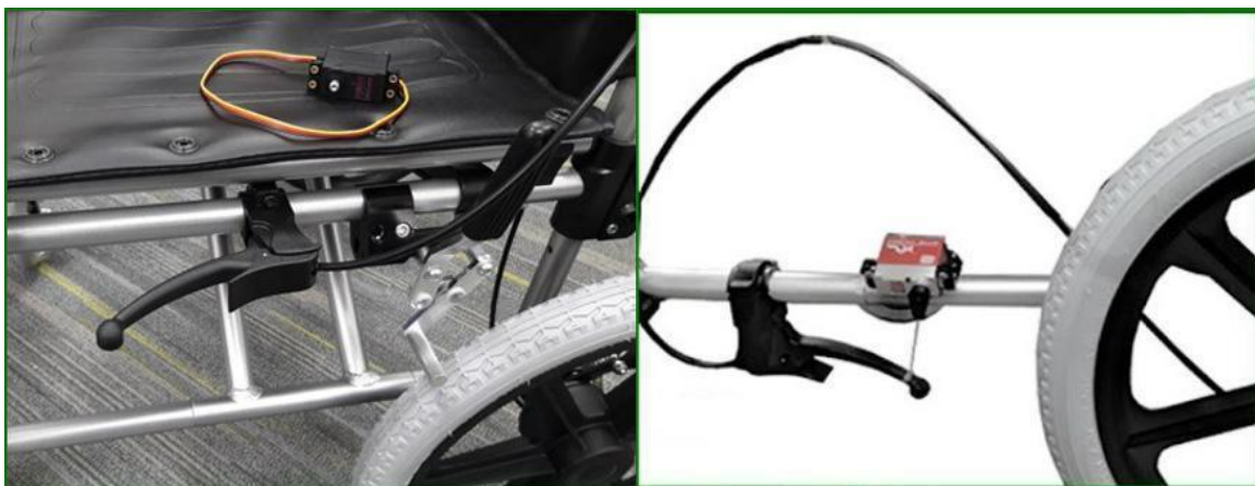
Figure 3.11 Wheelchair with repositioned brake lever and servo mounted and connected to repositioned brake lever.
